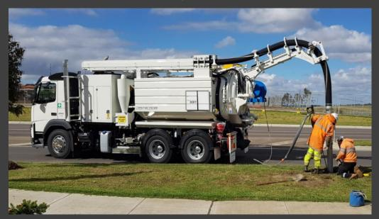
Our SV3700 brings you one of the best payloads in Australia on a 6x4 cab chassis. With a 3700 cubic metre per hour (2225cfm) Hibon Blower providing ideal performance for Vacuum Recovery or Hydro Excavation this is one of the most fuel efficient Industrial Services Vacuum Truck currently on the market.
