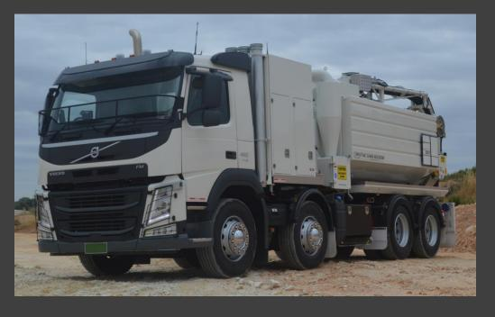
The SV4000 Hydro Excavation Vacuum truck from Spoutvac provides you with the best balanced unit in the industry. With a staggering 10,700kg payload and 4,000 cubic metre an hour 6" Liquid ring Vacuum system, the SV4000 is the most economical machine for large jobs. Mounted to a 5,100mm (European) wheel base FM11 Volvo the unit provides great handling and a turning circle to rival any 3 axle truck.
