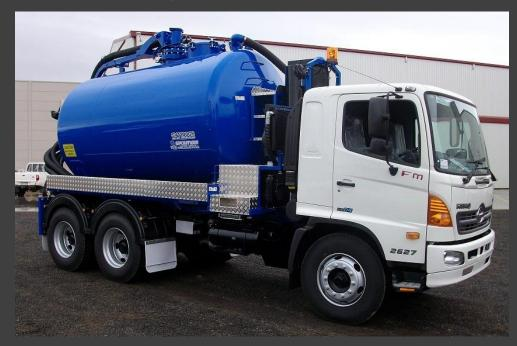
Available on FE Volvo, UD, Hino or Isuzu the GS150 is a basic liquid tanker with gravity or pressure discharge through a 100mm or 150mm Camlock connection or the 600mm manhole plate on the rear of the tank
