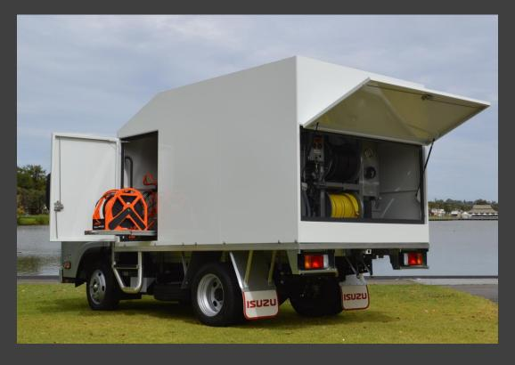
The Spoutvac 'Mini Rustler' Small Truck jetting unit has been designed for Australia's versatility, with a full galvanized frame aluminium clad body.
