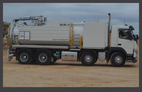
The SV6200 Hydro Excavation Vacuum truck from Spoutvac provides you with the best balanced unit in the industry. With a possible 10,000kg payload and 6,200 cubic metre an hour 8" Liquid ring Vacuum system, the SV6200 is the most economical machine for large jobs. Mounted to a 5,100mm (European) wheel base FM11 (450HP) or FM13 (460HP) Volvo the unit provides great handling and a turning circle to rival any 3 axle truck.
