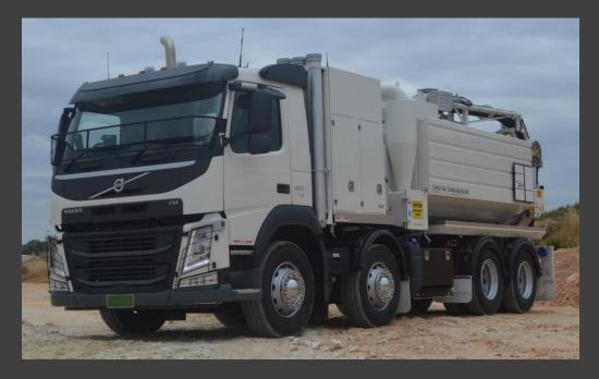
The SV4000 Hydro Excavation Vacuum truck from Spoutvac provides you with the best balanced unit in the industry. With a staggering 8,500kg payload and 4,000 cubic metre an hour 6" Liquid ring Vacuum system, the SV4000 is the most economical machine for large jobs. Mounted to a 5,100mm (European) wheel base FM11 Volvo the unit provides great handling and a turning circle to rival any 3 axle truck.
