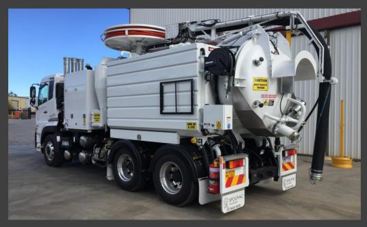
Configured as a turnkey package on the 6x4 UD or Volvo cab chassis, the Spoutvac combination truck combines hydraulic and belt drive systems that enable variable speed control between jetting and vacuum, providing better fuel economy by only using the power required to complete a job. With low maintenance, excellent weight distribution and the highest level of Health and Safety, the Spoutvac Combo provides optimum flexibility and efficiency.
