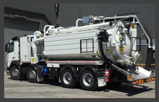
The SV6200 Hydro Excavation Vacuum truck from Spoutvac provides you with the best balanced unit in the industry. With a staggering 8,000kg payload and 6,200 cubic metre an hour 8" Liquid ring Vacuum system, the SV6200 is the most economical machine for large jobs. Mounted to a 5,100mm (European) wheel base FM11 Volvo the unit provides great handling and a turning circle to rival any 3 axle truck.
