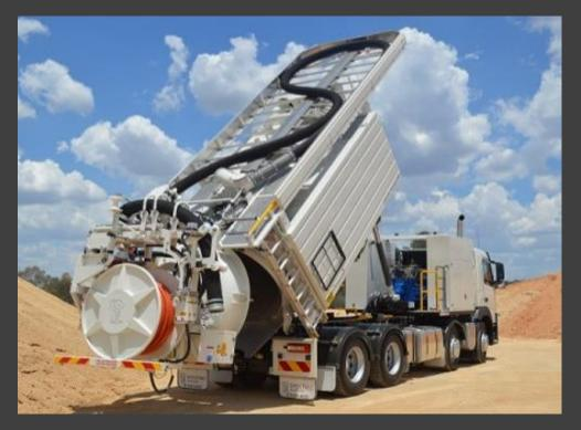
The Spoutvac 8x4 SV3750 Cassette combination truck comes with all the options of the traditional SV3750 Boom truck as well as having the extendable Vacuum hose option. Health and Safety is paramount with the Cassette system with its ability to lower and raise the vacuum hose in a pit with minimal lifting by the operator and its snake like design providing less blockages than other extendable vacuum hose systems.
