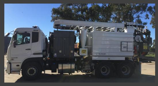
Configured as a turnkey package on the 6x4 UD or Volvo cab chassis, the Spoutvac combination truck combines hydraulic and belt drive systems that enable variable speed control between jetting and vacuum, providing better fuel economy by only using the power required to complete a job. With low maintenance, excellent weight distribution and the highest level of Health and Safety, the Spoutvac Combo provides optimum flexibility and efficiency.
