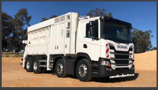
Spoutvac are now proud to offer the German built RSP product, known as the market leader in fan-operated suction excavation equipment. RSP have a great deal of experience in manufacturing mobile suction excavators or Non Destructive digging equipment. The RSP fan based technology can produce up to 42,000 m3/h or 24,720 cfm or air with a vacuum pressure of 11.8hg making it the most powerful vacuum unit available in Australia.
