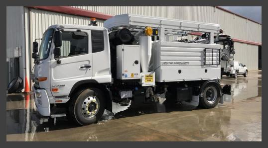
The Spoutvac SV2000 4x2 Cassette combination truck comes with all the options of the traditional SV3750 Cassette Unit only on a smaller frame. Health and Safety is paramount with the Cassette system with its ability to lower and raise the vacuum hose in a pit with minimal lifting by the operator and its snake like design providing less blockages than other extendable vacuum hose designs.
